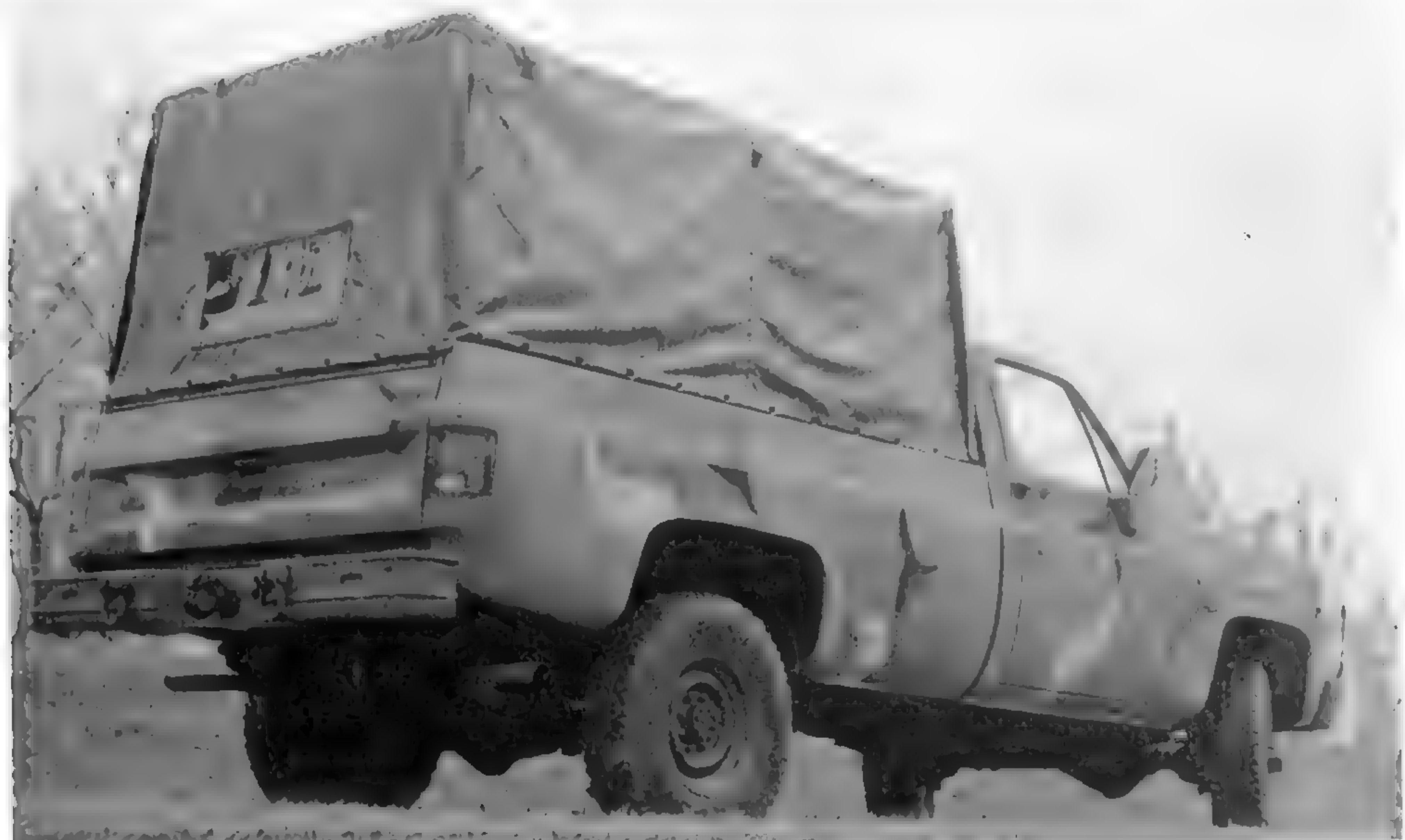
The pintle hook of the M1008 was mounted on a standard civilian step bumper. The front and rear shackles are attached to the frame. (U.S. Army photo)
